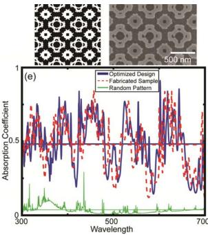
The optimized structure achieves a broadband absorption efficiency of 48.1% and more than 3fold increase over the Yablonovitch limit [2].
