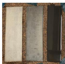
Tensile specimens manufactured using ASTM-D3039 standards.
