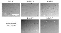
•Failure caused by largest inclusion •Optimal Y content in order to minimize largest inclusion size
